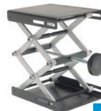
Raises and lowers sample vessels to a stationary probe as needed.
