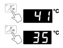
Display and adjustment of over-/undertemperature:
