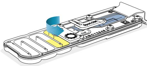
7 Remove all fluid from the waste channel through waste port 1 using a P1000 pipette.
