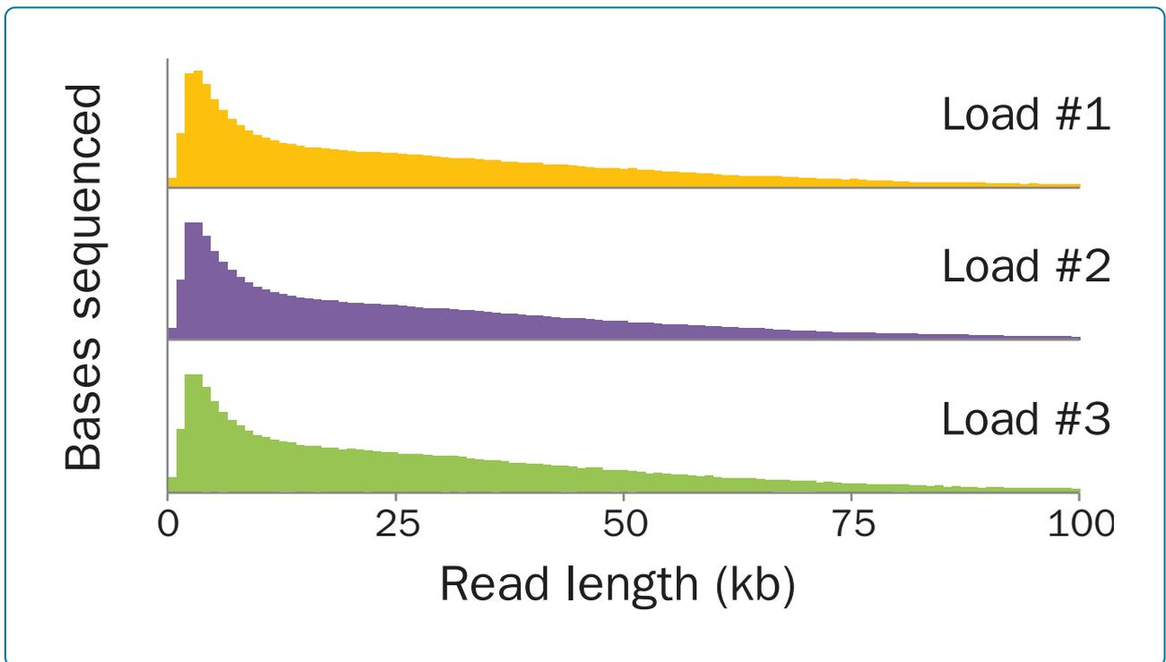
**Figure 4.** Effective inactivation of the DNase I prevents read length deterioration in the experiments after a nuclease wash is performed. In this example, the read length of the *Gallus gallus* library was recorded before the first wash (load #1) and then again after the first and second washes (load #2 and #3, respectively). No decrease in read length is observed.
