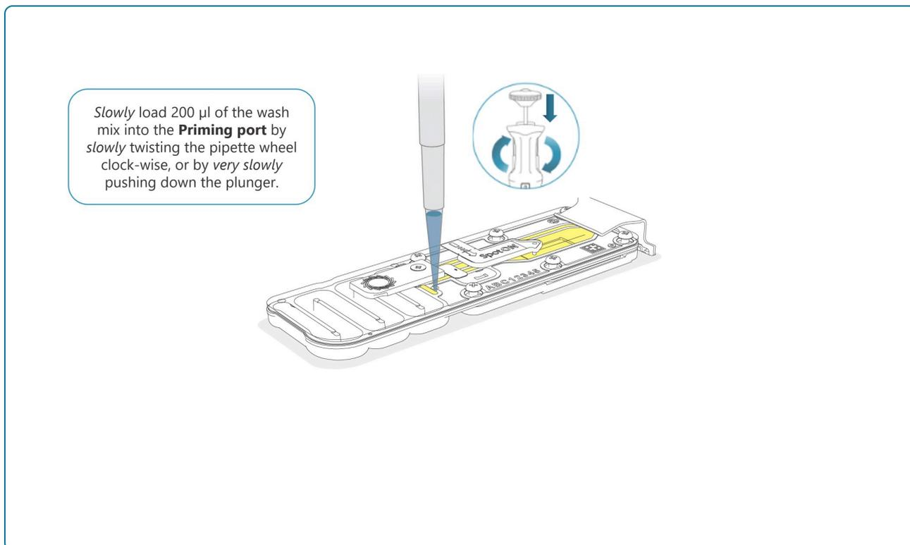
**11** Once the 5 minute incubation is complete, carefully load the remaining 200 µl of the prepared flow cell wash mix into the priming port, as follows:
