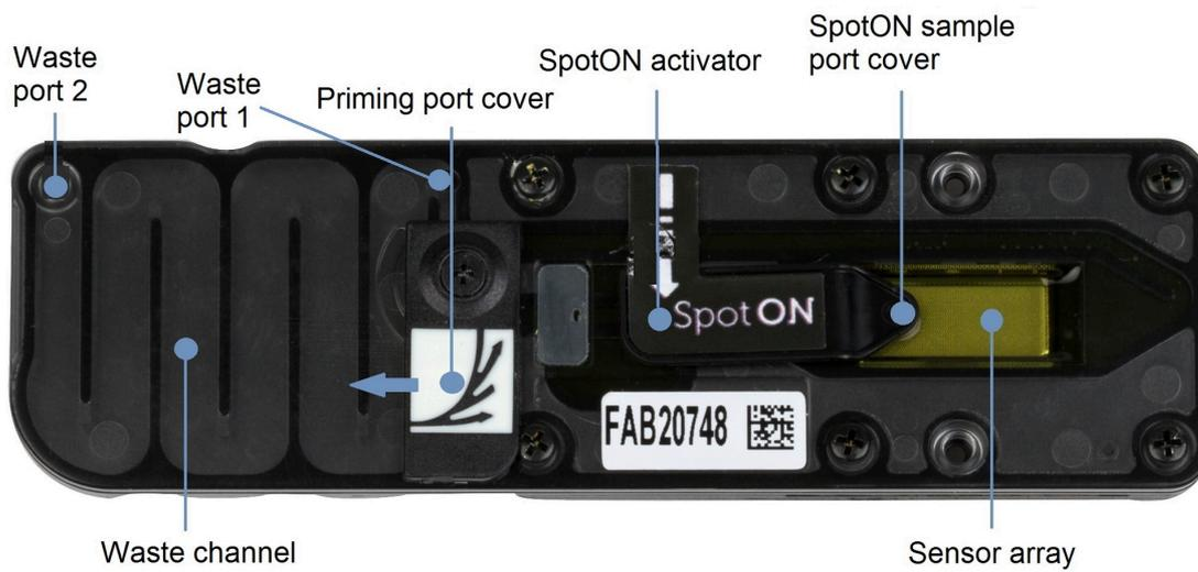
8 Slide the flow cell priming port cover clockwise to open.
