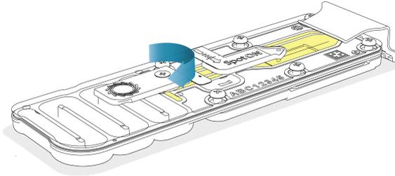
**4 After opening the priming port, check for a small air bubble under the cover. Draw back a small volume to remove any bubbles:**
