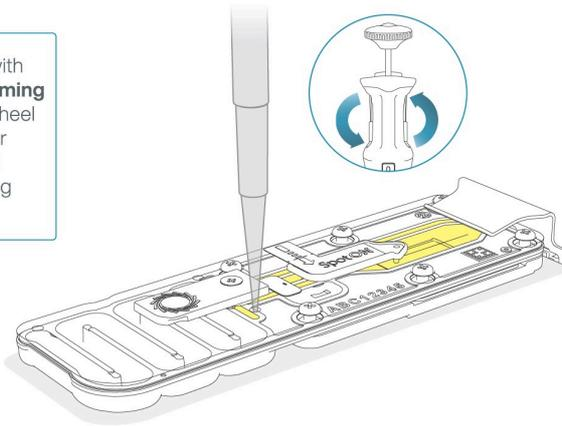
**5** Slowly load 800  $\mu\text{l}$  of the priming mix into the priming port, as follows:
