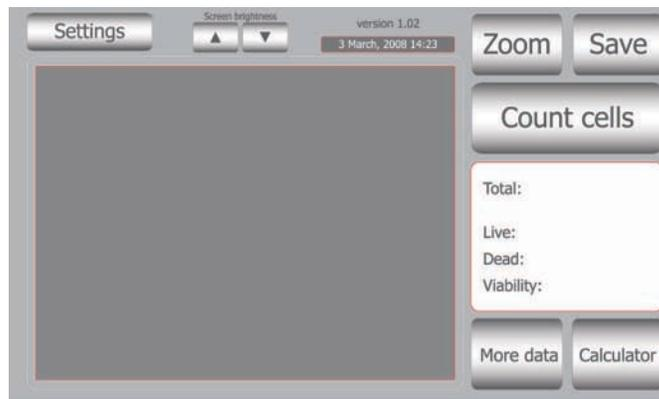
1.2 Press **Settings** and then press **Beads** to place the instrument into bead counting mode. Beads option becomes shaded gray.
