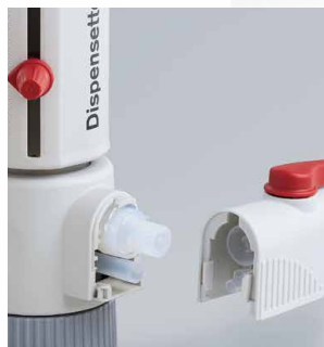
Valve system designed without seals
