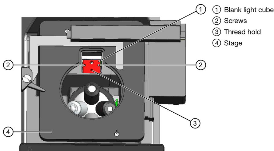
4. Using the light cube tool, loosen the two screws that attach the blank light cube to the instrument. You do not have to remove the screws.
