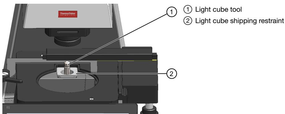
1. If installed, using the X-axis and Y-axis stage positioning knobs, move the mechanical stage back to obtain access to the light cube shipping restraint, which is centered under the back of the stage.
