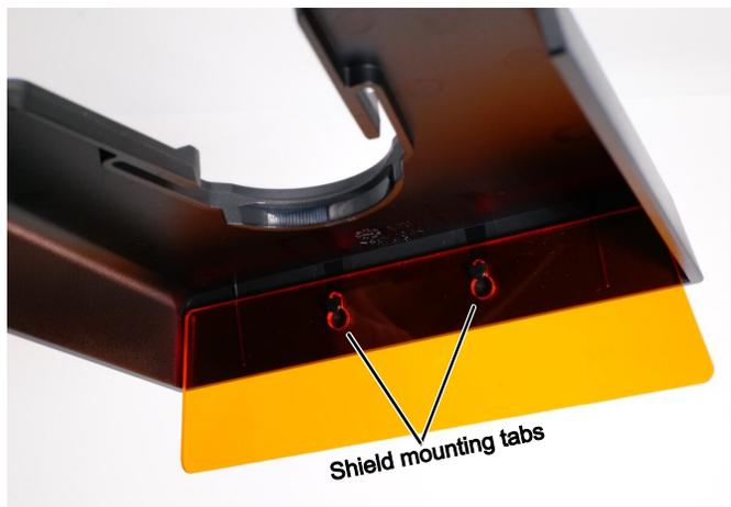
2. Attach the Condenser light shield to the Condenser using the groove in the Condenser barrel to clip it in place.
