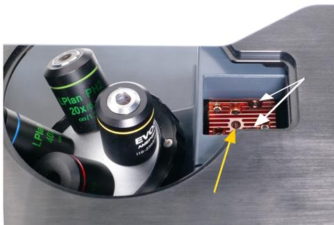
4. Use the light cube tool to loosen the two slotted screws (white arrows) that are flush with the ridges on the light cube.
