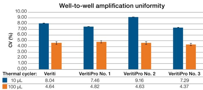
**Figure 2. Comparison of well-to-well amplification uniformity between one Veriti 96-Well Thermal Cycler and three VeritiPro 96-Well Thermal Cyclers at low (10 µL) and high (100 µL) reaction volumes.** The CV for each run was calculated using fluorescence intensity data after PCR in a MicroAmp Optical 96-Well Reaction Plate sealed with MicroAmp Clear Adhesive Film.
