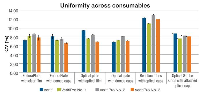
**Figure 4. Comparison of well-to-well amplification uniformity between one Veriti 96-Well Thermal Cycler and three VeritiPro 96-Well Thermal Cyclers using various combinations of PCR consumables including MicroAmp EnduraPlate and Optical plates.** The CV for each run was calculated using fluorescence intensity data from low-volume (10 µL) reactions.
