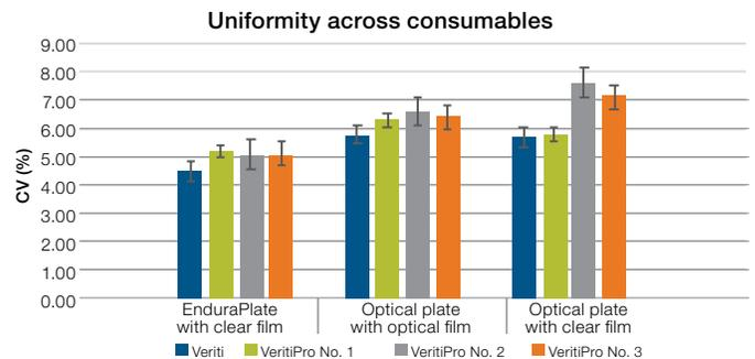
**Figure 5. Comparison of well-to-well amplification uniformity between one Veriti 384-Well Thermal Cycler and three VeritiPro 384-Well Thermal Cyclers using various combinations of MicroAmp EnduraPlate and Optical plates with various films.** The CV for each run was calculated using fluorescence intensity data from low-volume (5 µL) reactions.
