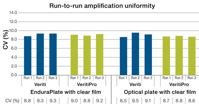
**Figure 6. Comparison of run-to-run amplification uniformity between Veriti 96-Well and VeritiPro 96-Well Thermal Cyclers on MicroAmp EnduraPlate and Optical plates with clear film.** The CV for each run was calculated using fluorescence intensity data after PCR in 10  $\mu$ L reactions.
