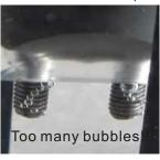
5. Stir the probe gently in the sample to create a homogenous sample. Allow a few seconds to reach temp. equilibrium. (Wait about 15 minutes can get a stable reading) 6. Press "Local" to freeze current readings. The text "H" will appear on the LCD. Press "HOLDCAL" again to release.
