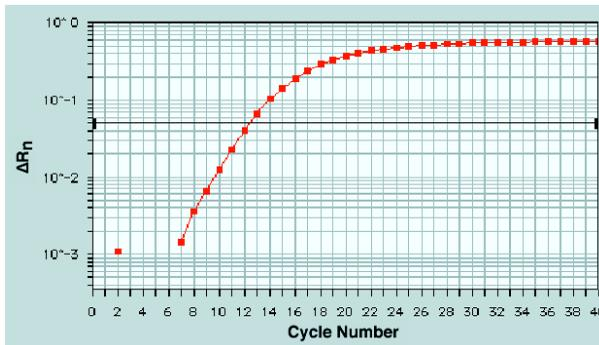
**Figure 4-4** Amplification plot with correct baseline (logarithmic ordinate)
