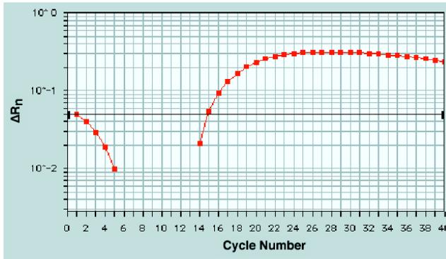
**Figure 4-2** Amplification plot with incorrect baseline (logarithmic ordinate)
