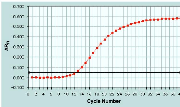
**Figure 4-3** Amplification plot with correct baseline (linear ordinate)
