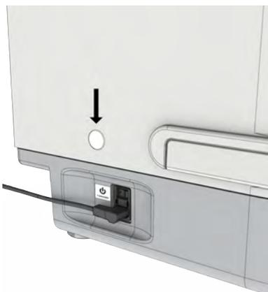
2. Remove the blanking plug from the entry point using a small flat screwdriver.
