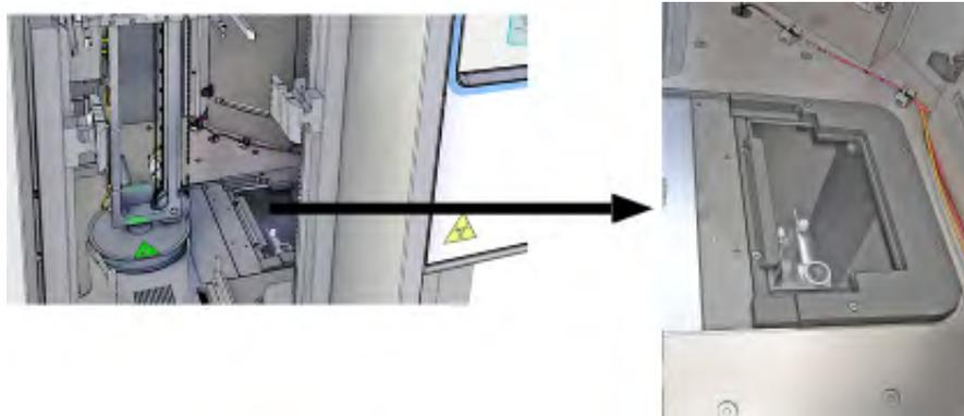
**Figure 24** Location of glass plate on the internal OptiRead™ module
