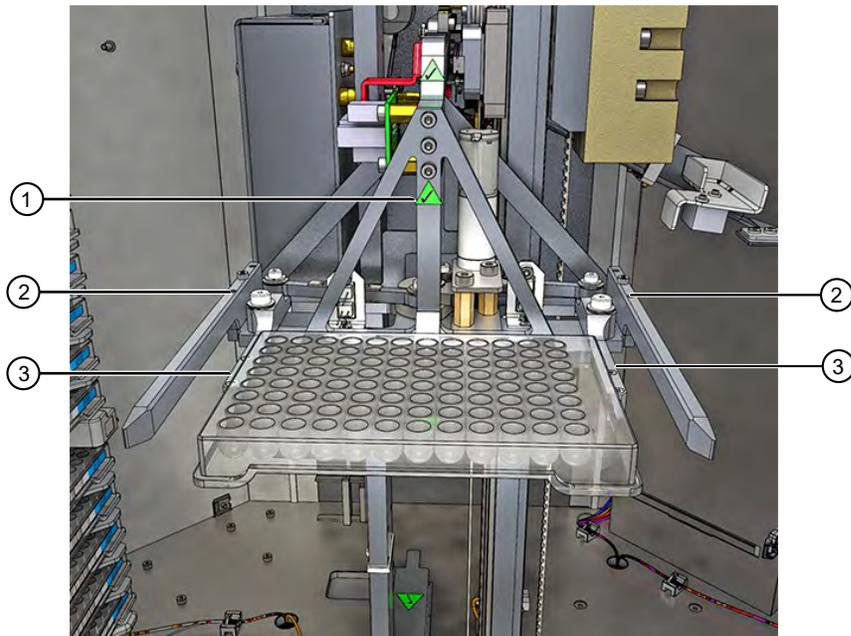
**Figure 36** Narrow and wide arm grippers
