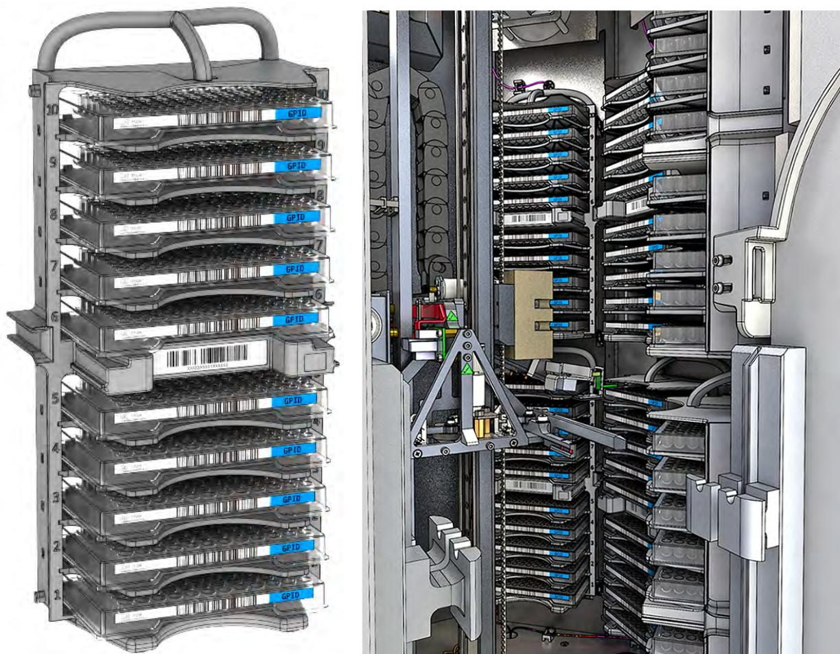
Figure 9 Racks, free-standing (left) and mounted inside the ARIS HiQ™ system (right)
