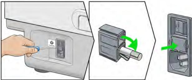
Figure 22 Replacement of the fuse in the power inlet
