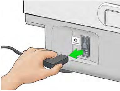
Figure 27 Disconnect the power cable from the instrument
