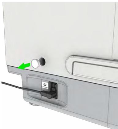
3. Insert the temperature probe through the slitted bung provided with the instrument, then through the entry point.
