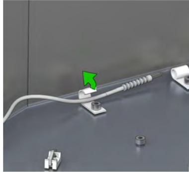
7. Arrange the cable so the probe head and terminating cable are located as shown in the following picture.
