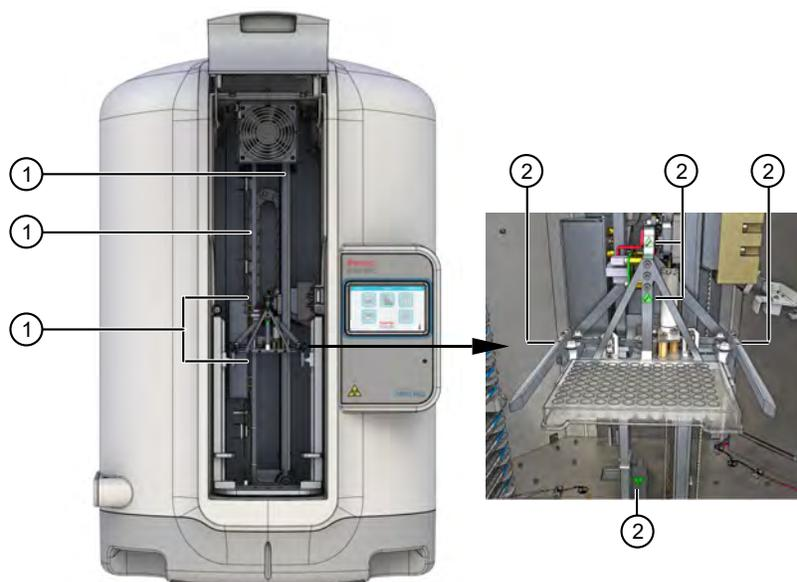
**Figure 35** Transfer arm assembly
