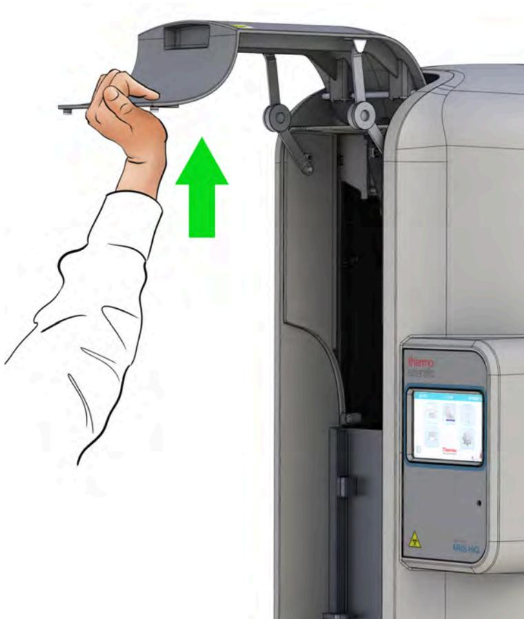
Figure 32 Access door to the incubation chamber
