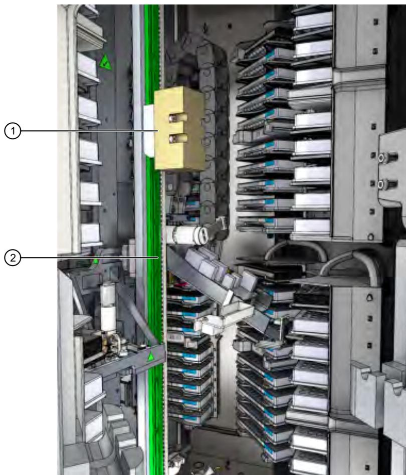
**Figure 25** Counterbalance weight and guide
