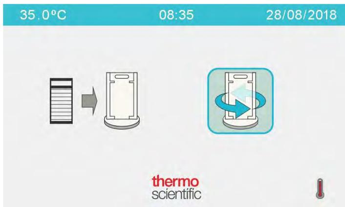
After the empty utility rack is rotated to the inside of the turntable, the system scans the rack for plates, scans plate barcodes, updates the plate inventory, then the **System Status** screen is displayed with updated indicators.
