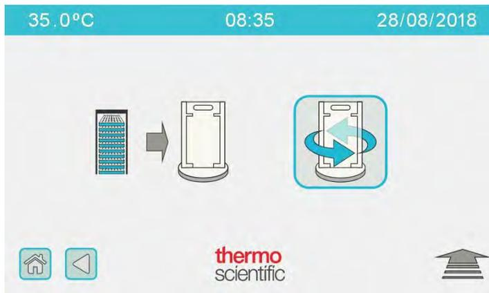
The rack rotates to the inside of the system. The robotic arm moves the rack to the inside wall of the system.
