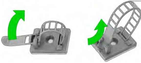
2. Unclip the probe cable from the 5 clips located on the baseplate and the back wall of the instrument.
