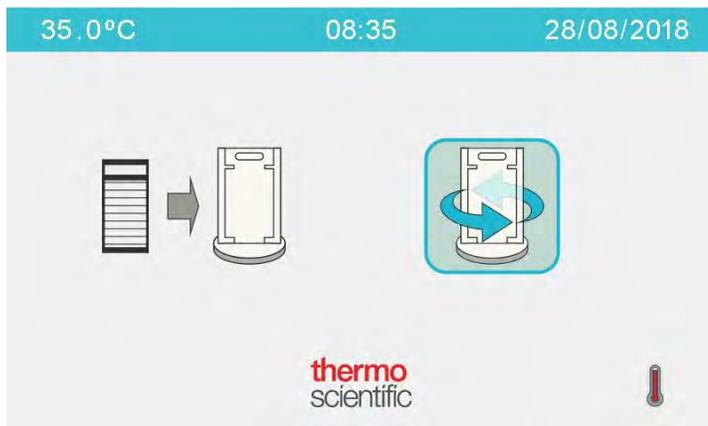
The empty rack is moved to the inside of the turntable, then the robotic arm places completed plates in the rack.
