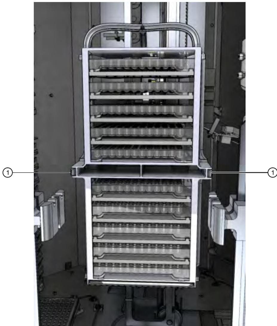
Figure 37 Wide arm gripper holding a rack
