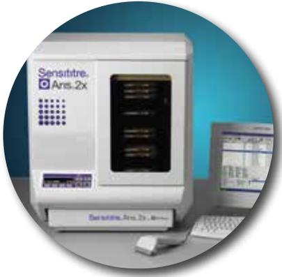
**Thermo Scientific Sensititre ARIS 2X System.** The ARIS™ 2X System is a fully automated, benchtop incubating and reading system that reduces workload and facilitates efficient workflow. It can accommodate 64 MIC, breakpoint or identification plates, for a combination of 192 possible tests on a single instrument.
