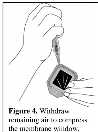
**Figure 4.** Withdraw remaining air to compress the membrane window.
