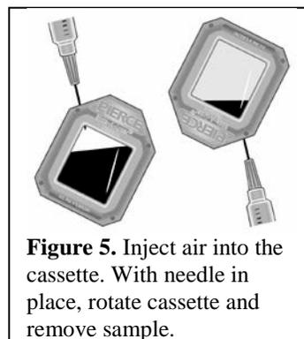
**Figure 5.** Inject air into the cassette. With needle in place, rotate cassette and remove sample.
