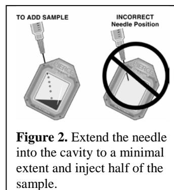
**Figure 2.** Extend the needle into the cavity to a minimal extent and inject half of the sample.
