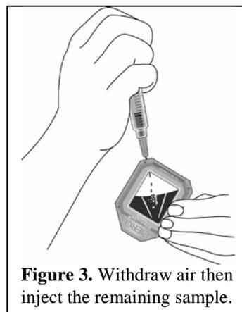
**Figure 3.** Withdraw air then inject the remaining sample.
