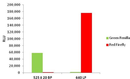
**Figure 3. Specificity analysis of the two luciferase emissions.** Green *Renilla* luciferase was measured using a 525±20nm BP filter and red firefly luciferase was measured using a 640nm LP filter on a Thermo Scientific™ Varioskan™ Luminometer.
