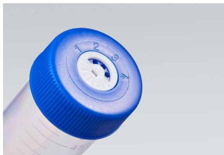
Adjustable 4-level vented cap allows for gas exchange and air circulation. This product design is ideal for high-throughput mammalian protein expression screening and cell line development.
