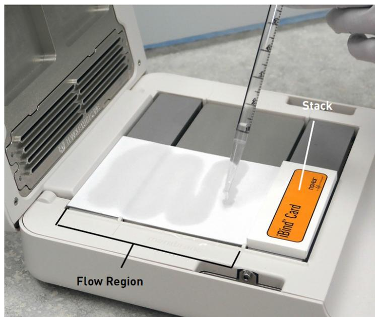
7. Pipette 1 mL of 1X iBind™ Flex/ iBind™ Flex FD Solution so that it pools at the center of the membrane region on the iBind™ Card.
