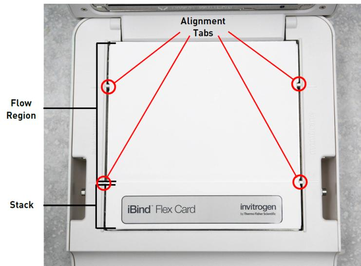
The iBind™ Flex Card is placed on the iBind™ Flex Western Device so that it fits between the alignment tabs with the stack facing the front of the device.
