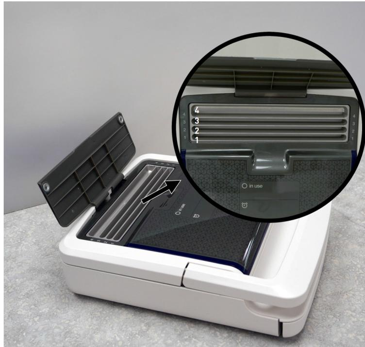
2. Close the Well Cover and write the start time of incubation on the lid of the iBind™ Flex device.
