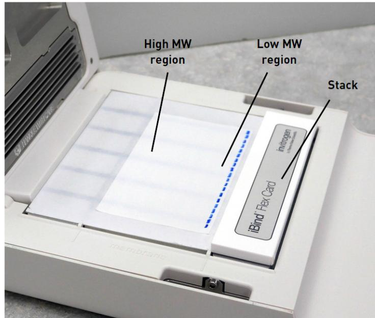
2. Use the Blotting Roller to firmly roll membrane on the iBind™ Flex Card, to ensure good contact and remove any air bubbles.
