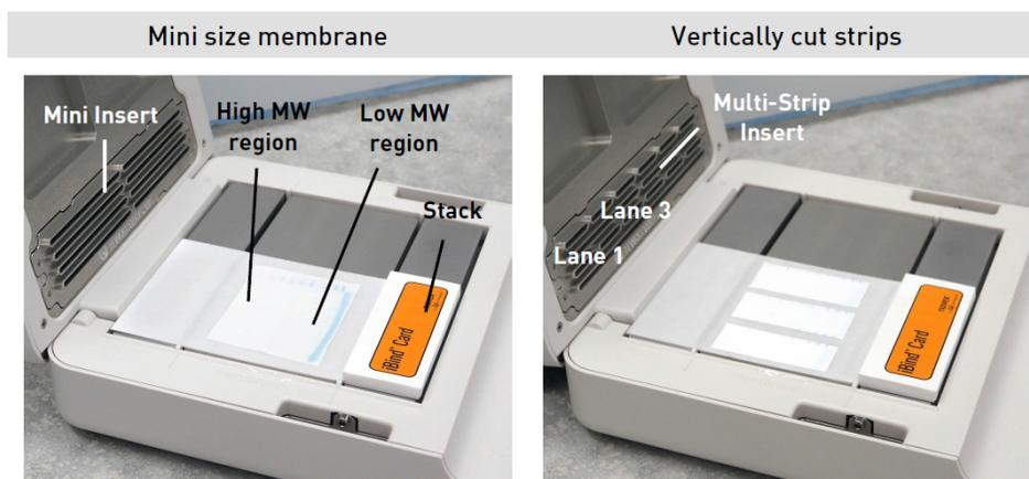
2. Use the Blotting Roller to firmly roll membrane on the iBind™ Card to ensure good contact and remove any air bubbles.
