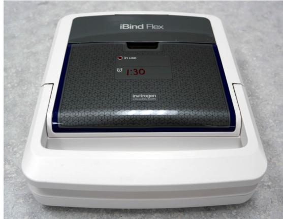
The iBind™ Flex Western Device consists of a metallic stage made up of three sections. The front and rear sections of the stage are spring plates designed to apply specific amounts of pressure on an iBind™ Flex Card placed on the stage when the lid of the device is locked.
