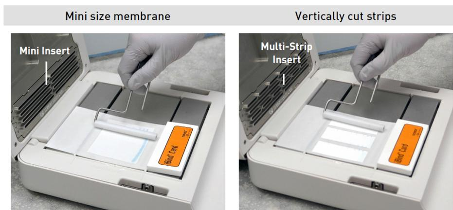
3. Ensure the iBind™ Card is flush against the alignment tabs, and that the membrane is within the boundaries of the membrane region. **No part of the membrane should be directly under the well insert.**
