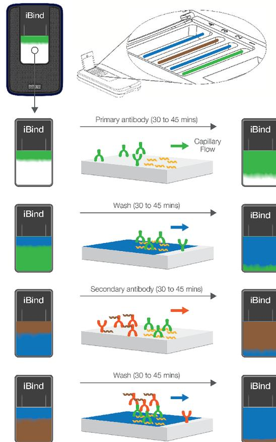
Figure 1 Sequential lateral flow technology employed by the iBind™ Flex Western System.
