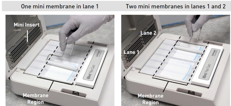
3. Ensure the membrane(s) are aligned with the lane(s) and within the boundaries of the membrane region. **Ensure no part of the membrane is directly under the Mini Insert.**
