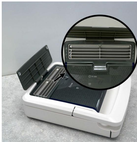
2. Close the Well Cover and write the start time of incubation on the lid of the iBind™ Flex device.
