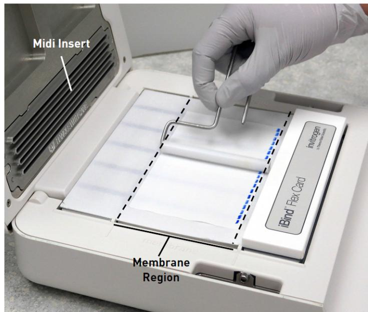
3. Make sure the membrane is within the boundaries of the membrane region. **Ensure no part of the membrane is directly under the Midi Insert.**
