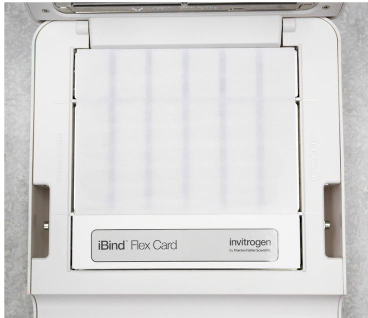
When the flow region is wet with solution, lines appear on the iBind™ Flex Card to assist in alignment of mini-sized or vertically cut strip membranes with lanes.
