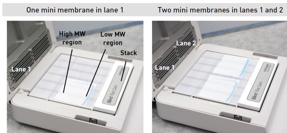
2. Use the Blotting Roller to firmly roll membrane on the iBind™ Flex Card, to ensure good contact and remove any air bubbles.
