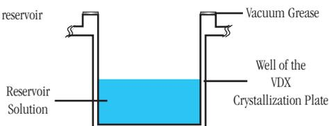
2. Using a clean pipet tip, pipet 1 ml of Crystal Screen reagent 1 into reservoir A1. Discard the pipet tip, add a new pipet tip and pipet 1 ml of Crystal
