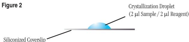
4. Pipet 2 µl of Crystal Screen reagent 1 from reservoir A1 into the sample droplet and mix by aspirating and dispensing the droplet several times, keeping the tip in the drop during mixing to avoid foaming. See Figure 2.
