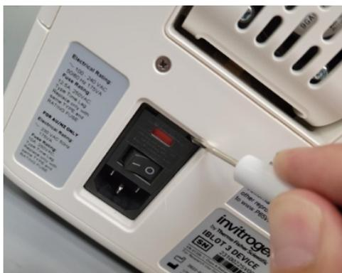
4. Using the screwdriver, gently pry out the red fuse holder.
