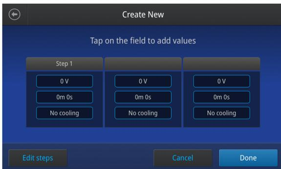
3. Tap the desired field and use the keyboard to enter the appropriate values for **Volts** (5 V to 35 V), **Time** (1 min to 25 mins), **Cooling fan speed** (No cooling, Low cooling, Med. cooling, or Max. cooling) for step 1. Repeat the procedure as necessary for step 2 and step 3.
