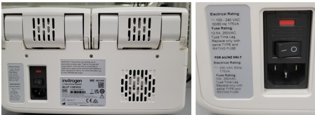
3. Using a small flat-head screwdriver, pry open the fuse door. The door will fall forward from the device.
