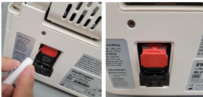
5. Remove each fuse from its fuse holder and inspect it for damage. Black carbon inside the glass typically indicates a defective fuse.
