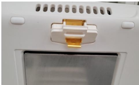
3. Using the screwdriver, unscrew the 2 screws holding the contact. Discard the old screw and contact.
