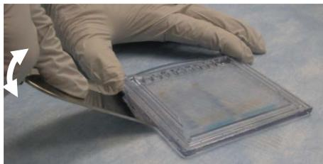
4. Rotate the cassette and repeat Steps 2–3, until the two plates are completely separated.
