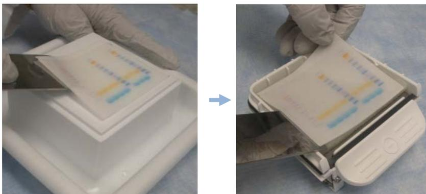
5. Wet the surface of the gel with 1X Transfer Buffer and remove any bubbles with the Blotting Roller.
