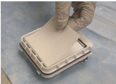
8. Place a pre-soaked sponge pad onto the filter paper. Remove any bubbles with the Blotting Roller.
