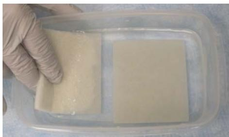
Leave the sponge pads in the container of 1X Transfer Buffer until you are ready to use them to assemble the blot sandwich.
