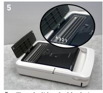
5. Close the lid and add solutions sequentially to the wells starting with well 1 (see Table 1 for solutions). Close the well cover.
