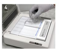
4. Use the Blotting Roller to firmly roll membrane on the iBind™ Flex Card to ensure good contact and remove any air bubbles.
