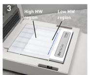
3. Place the membrane on top of the pooled solution with the **protein-side down**, and the low molecular weight region closest to the stack.
