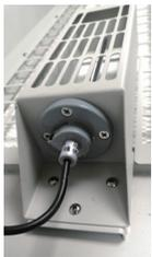
The hot-ball anemometer monitors the wind speed in the working area and exhaust area of the safety cabinet in real time, then compares this with the standard wind speed. The rotating speed of the fan is adjusted through the microprocessor system to maintain the constant wind speed of the safety cabinet.
