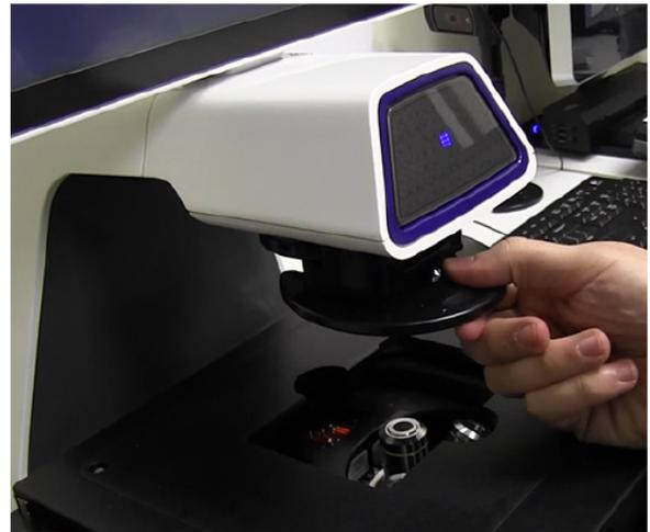
3. Secure the UV light shield mount to the top of the condenser light shield using the two screws and 2 mm hex key supplied with the UV shield assembly (not the protruding screws on the mount).
