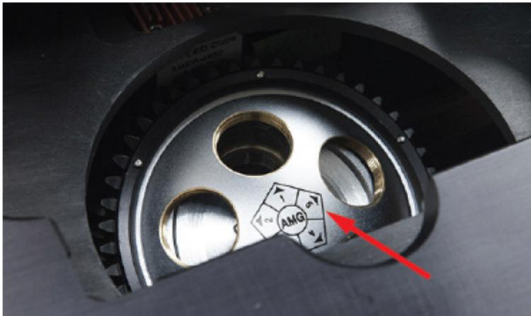
2. Screw the new objective into the open position in the objective turret. Note the part number of the objective and the turret position. In this example, the new objective is installed into the turret position 5.
