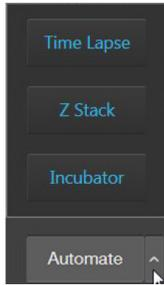
**Time Lapse:** Opens the **Time Lapse** tool, which allows you to create and run time lapse routines to capture images at given intervals over a time period based on your specifications.
