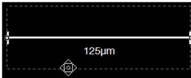
6. To adjust the length of the scale bar, hover your pointer over the scale bar until a bounding box appears, then the click left or right side of the box and drag the box to the desired length. You can adjust the length by pre-fixed increments based on the objective magnification.
