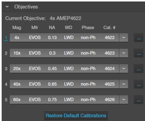
2. Find the newly installed objective in the **Objectives** list for the corresponding turret position.
