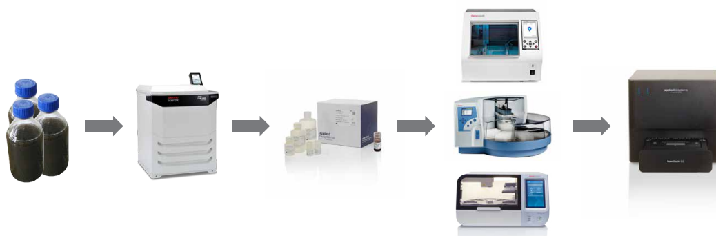
Figure 2. End-to-end workflow of wastewater sample testing with the QuantStudio Absolute Q dPCR System. Wastewater samples are clarified by centrifugation, followed by an optional magnetic bead-based virus enrichment step. Extraction reagents and samples are then loaded onto one of three KingFisher systems (shown are the Thermo Scientific™ KingFisher™ DuoPrime, Flex, and Apex Purification Systems). Eluates are combined with master mix and assay(s), loaded into the QuantStudio Absolute Q MAP16 dPCR plate, and run on the QuantStudio Absolute Q dPCR system.
