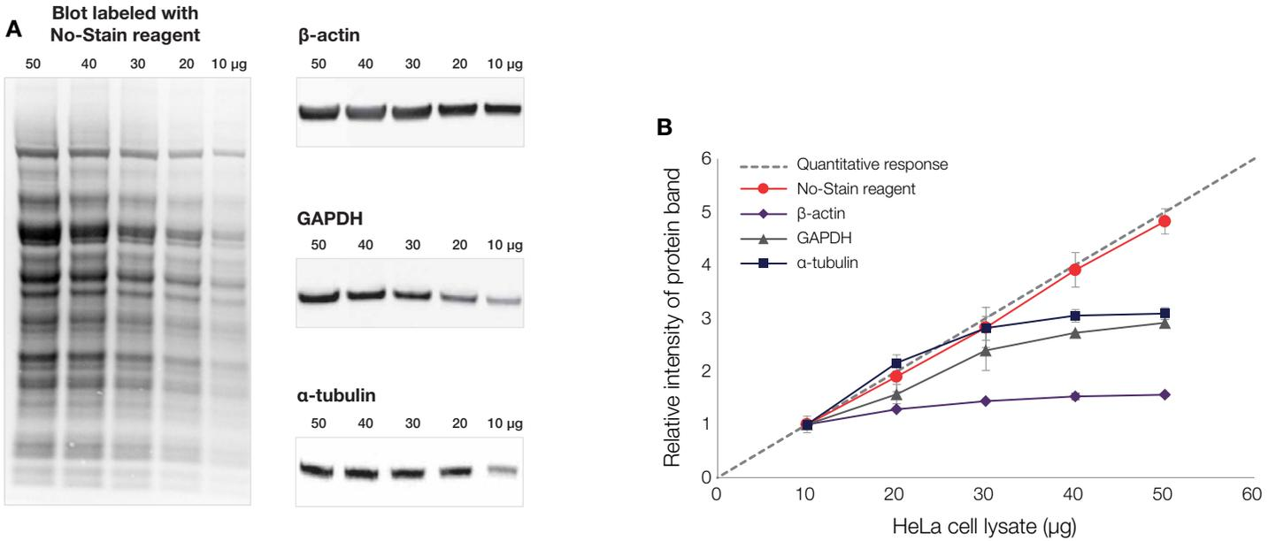
**Figure 21. Signals from housekeeping proteins become saturated as protein load increases. (A)** Western blots of HeLa cell lysates labeled with No-Stain reagent or  $\beta$ -actin, GAPDH, or  $\alpha$ -tubulin probes. **(B)** Densitometric analysis of the blots in panel A. The signal from total protein in the HeLa cell lysate labeled with No-Stain Protein Labeling Reagent stays linear with increasing protein load.
