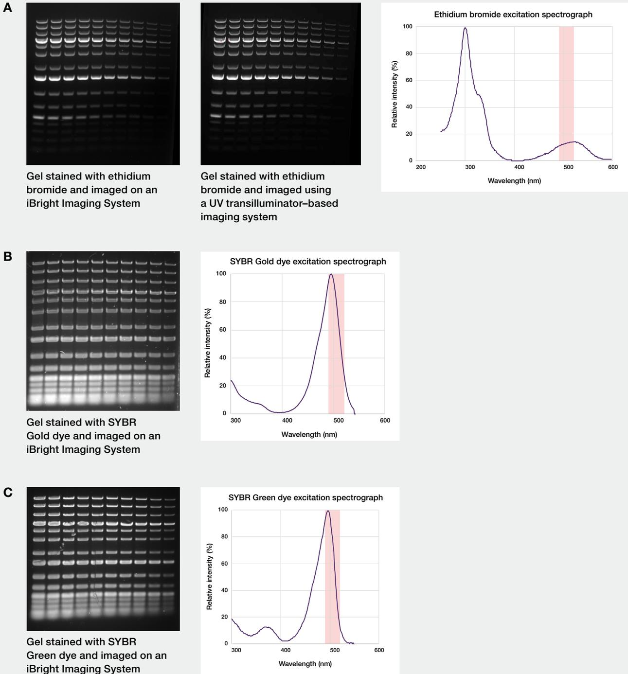
**Figure 23. The iBright green LED transilluminator effectively excites common DNA stains.** Excitation spectrographs of (A) ethidium bromide, (B) SYBR Gold dye, and (C) SYBR Green dye (purple lines). The 490–520 nm emission range of the iBright transilluminator is indicated by the light red boxes.
