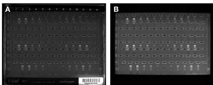
**Figure 10. Imaging with iBright Tray Adapters helps prevent fluorescence emitted by the E-Gel cassette barcode and label from interfering with the algorithm used by Smart Exposure technology.** Images of an E-Gel 96-well agarose gel captured (A) without and (B) with an iBright Tray Adapter.
