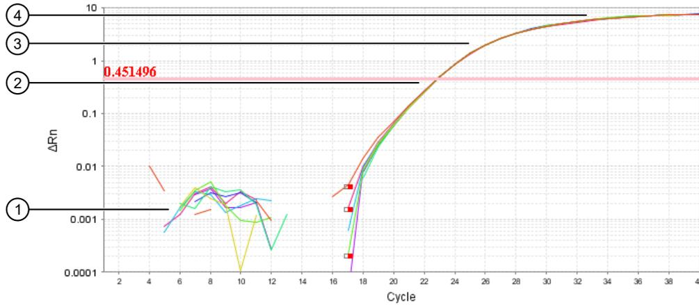
**Figure 4 Typical Amplification Plot**
