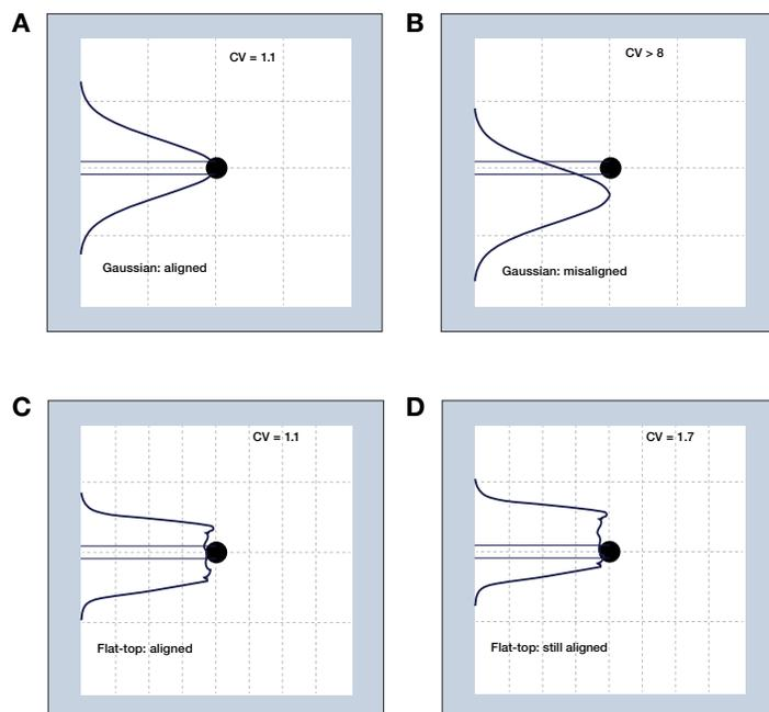
**Figure 2. Emission profile of lasers used in flow cytometers.** (A) Gaussian laser profile with proper alignment, (B) Gaussian laser profile with misalignment, (C) flat-top laser profile with proper alignment, and (D) flat-top laser profile still in proper alignment.
