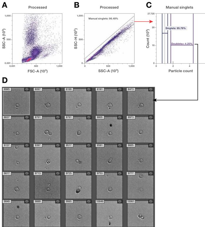
**Figure 9. Gating errors in traditional flow assays are highlighted with images. (A)** Human blood **(B)** gated for singlets using traditional scatter -A vs. -H approach, which includes **(C)** >4% of events with two or more cells. **(D)** The Image View Gallery is available to rapidly visualize these and other gating inaccuracies.
