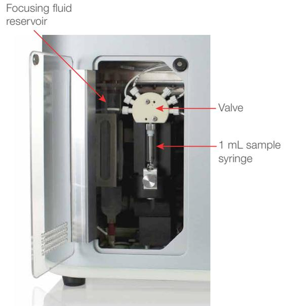
**Figure 3. Positive-displacement syringe pump.** The syringe is easily removed for cleaning or replacement in this example from the Invitrogen™ Attune™ NxT Flow Cytometer.
