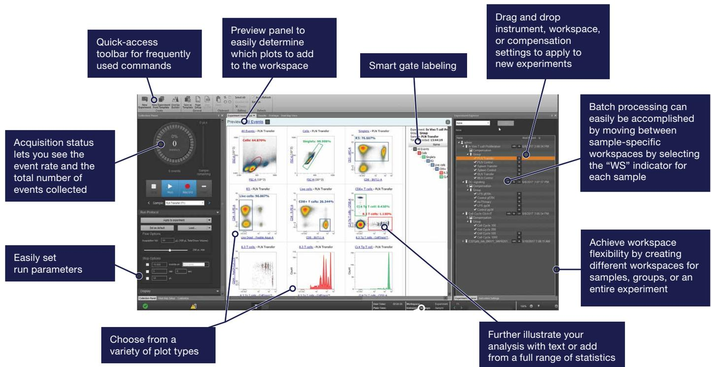
Figure 18. Intuitive, user-friendly software interface with a familiar workflow. A typical Attune NxT workspace interface is shown.
