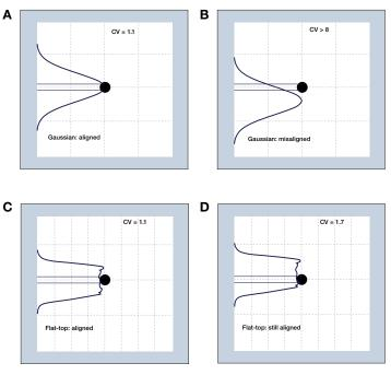
Figure 2. Emission profile of lasers used in flow cytometers. (A) Gaussian laser profile with proper alignment, (B) Gaussian laser profile with misalignment, (C) flat-top laser profile with proper alignment, and (D) flat-top laser profile still in proper alignment.
