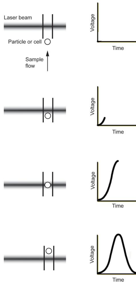
**Pulse measurement** The analog signal from the detectors are amplified and relayed to the 16-bit analog-to-digital converter (ADC), which samples the signals at a rate of up to 20 MHz, converting the continuous signal into digital data up to 35,000 events per second.
