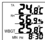
2. Press "**MIN/MAX**" key again, "MAX" appears on LCD left bottom. The maximum TA, RH% and WBGT(or DP, or EXT) appear on LCD.
