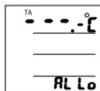
4. TA High alarm limit setup (adjustable range:-10.0~70.0°C):
