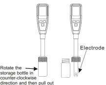
direction and then pull out the bottle completely to expose the electrode.
