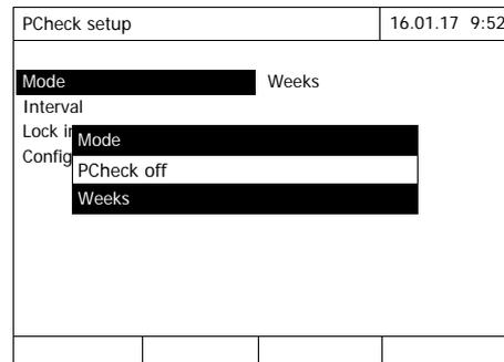
Select and confirm *Weeks*. PCheck is switched on. The *Interval* setting indicates *Weeks* as the interval unit.
