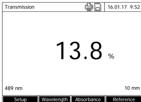
5 Using [Absorbance] <-> [Transmission], switch over the display from Absorbance to Transmission or vice versa.
