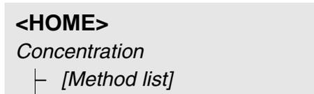
The list of methods is displayed. The methods are sorted by method number. The arrows ▼ or ▲ on the right edge indicate that the list comprises more methods further up or down.
