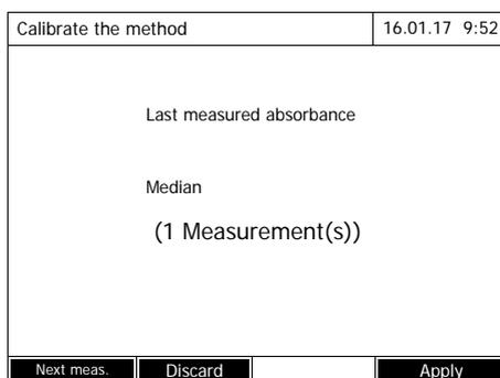
**6** If necessary, make additional single measurements for the median value formation with *[Next meas.]* or discard the last single measurement with *[Discard]*.
