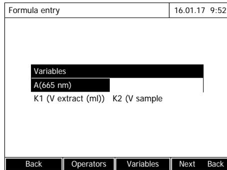
**11** Use [Variables], <▲><▼> <◀><▶> and <START-ENTER> to select Variable A<sub>665 nm</sub> and confirm. The current status of the formula is displayed.
