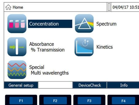
Press the function key <F1> (*[Setup]*). The *General setup* submenu pops up.
