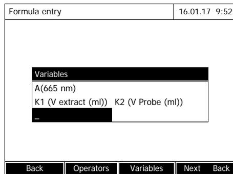
**12** Using [Variables], <▲><▼> <◀><▶> and <START-ENTER> select underscore (\_) The input field pops up where you can enter an index for the measurement, e.g. 2 for the second measurement at this wavelength. Confirm the index entered. The current status of the formula is displayed.
