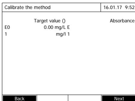
**8** Select all fields consecutively in the column *Absorbance* and start the corresponding measuring procedure with **<START-ENTER>**.
