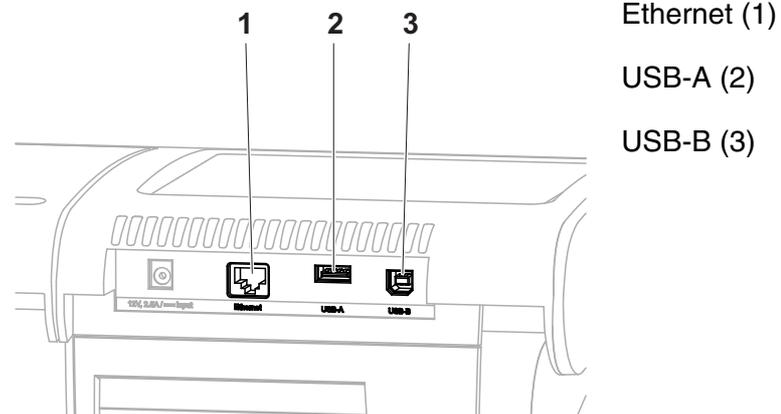
Figure 3-1 Communication interfaces on the rear panel
