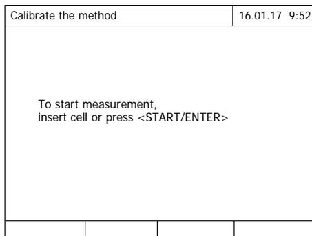
**5** Insert the cell with the corresponding standard or reagent blank value (for E0).
