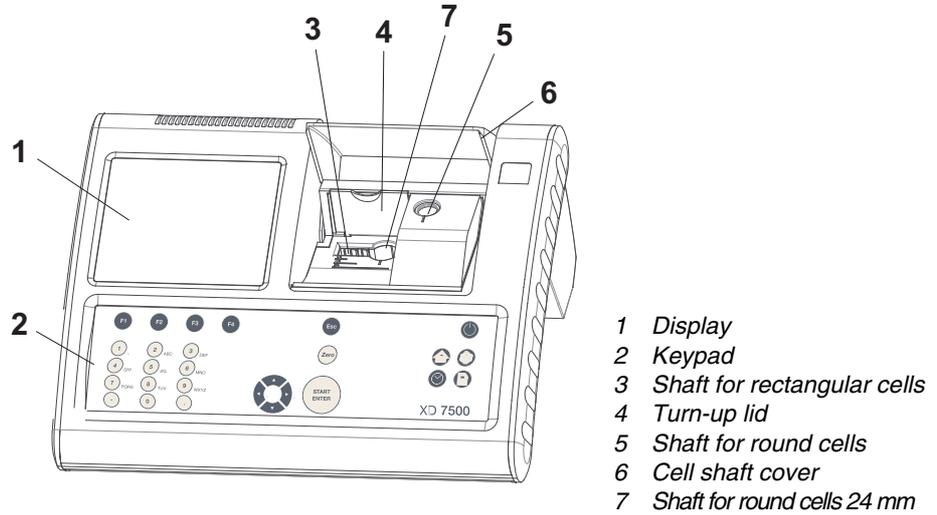
Figure 2-1 Front of the instrument with operating elements
