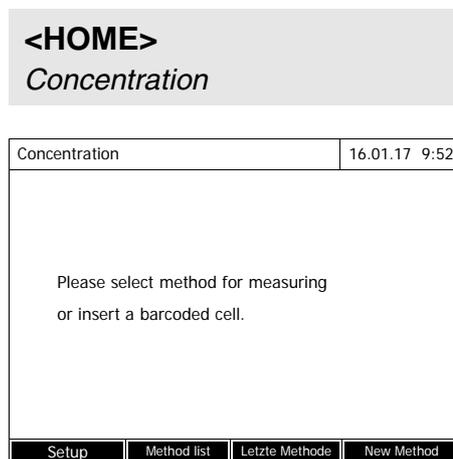
Inserting a cell with barcode starts a measurement.
