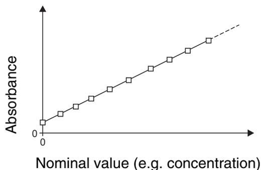
Figure 4-1 Example of a linear calibration function after a 10-point calibration
