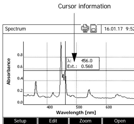
The cursor consists of a horizontal and a vertical line, which cross at a point of the curve. A box displays the x and y values of the curve point.
