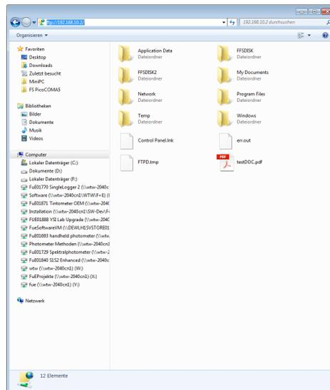
In Windows-Explorer on the PC, enter ftp://IP-address. The folders stored on the photometer are displayed.
