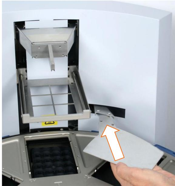
**Figure 9.** Inserting the shield plate
