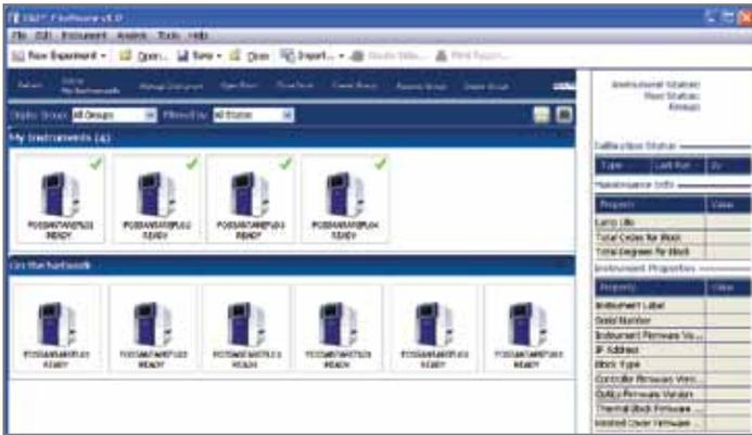
**With the ViiA™ 7 System, up to four instruments can be remotely controlled and precisely monitored in real time.** You can even review detailed run statistics and other vital information remotely and receive status notifications by email. Up to 15 instruments can be networked to provide basic instrument status information from any networked computer.
