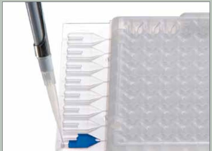
**TaqMan® Array Micro Fluidic Card.** Streamlines reaction setup, does not require liquid-handling robotics, and provides standardization when screening selected panels of genes.
