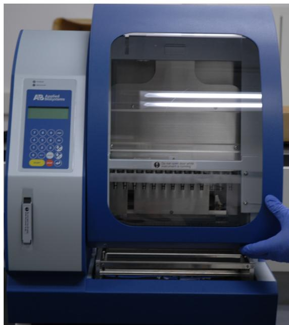
3. Load 13 empty reagent cartridges into the cartridge rack, then insert the loaded cartridge rack as described in “Load and insert the cartridge rack” on page 14.
