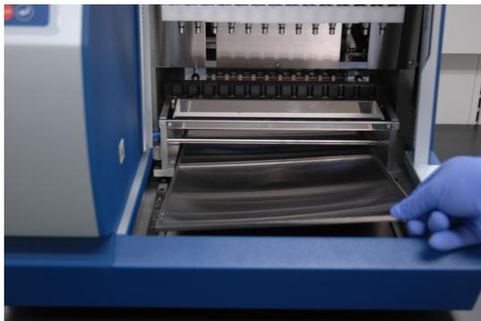
4. Insert the cartridge rack into the instrument.
