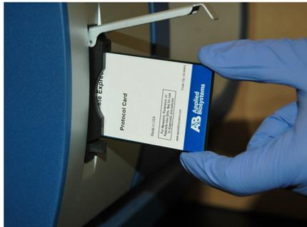
4. Push the card completely into the card slot, then close the card slot.
