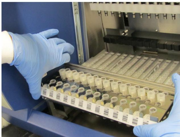
6. Ensure that you have inserted the cartridge rack and tip and tube rack correctly, then close the instrument door.
