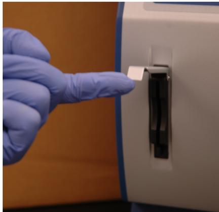
3. Insert the protocol card in the slot, with the arrow pointing toward the instrument and the label facing left.
