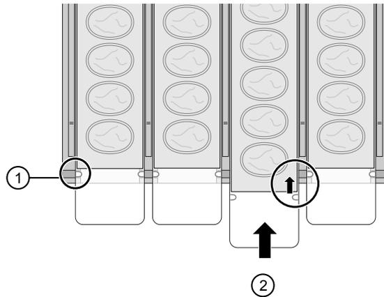
6. Insert the loaded cartridge rack into the instrument.
