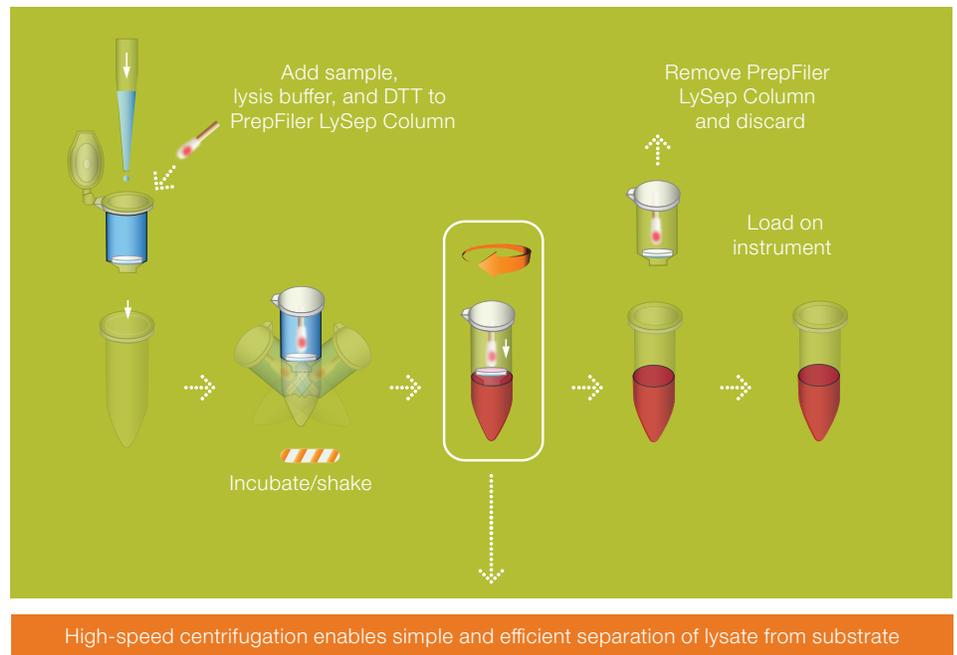
Figure 5. Improved method allowing users to easily perform lysis and effective substrate removal in a single-tube assembly.
