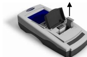
5– Place the selected standard in the sample chamber on the right hand side.
