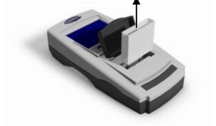
7 - Pour away the EC 2000 Zero solution in the cell then fill this Cell 2/3 full with the EC 2000 validation liquid.
