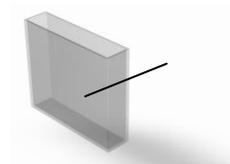
3 - Place the cell in the sample chamber of the EC 2000 Pt-Co, push to the left hand side.
