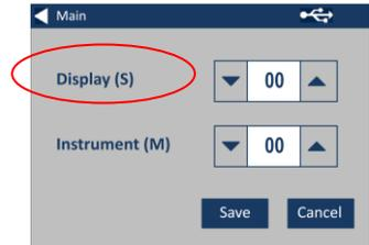
5b – Press the up and down arrows to set the time interval before the instrument shuts down after being inactive.
