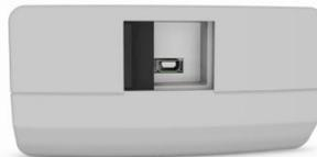
2 - Ensure the cable connector is inserted into the socket in the correct orientation. The symbol on the USB connector should be facing down.
