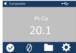
12 - Compare the result from the instrument to the value on the label of the validation liquid, to check it is within the specified tolerances.
