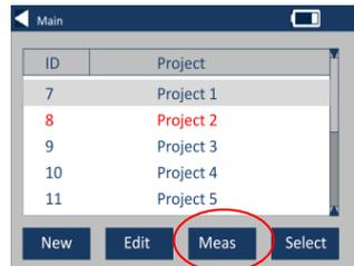
23 – This will bring up a list of the measurements stored for this project. If the tolerance limits are switched on (step 7), the results will be displayed as in the tolerance column (see page 15)
