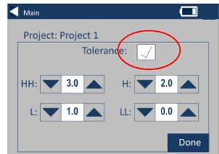
9 – To change the tolerance values, use the appropriate up and down arrows. Select Done when complete.
