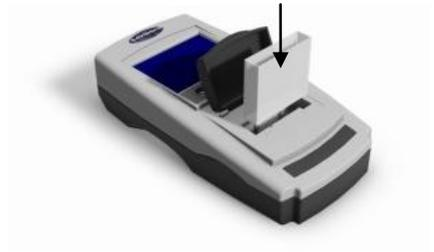
9 - Close the sample lid and press the test key.
