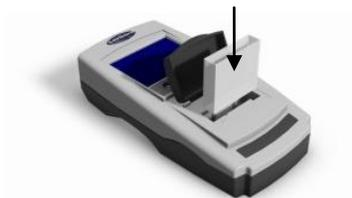
4 - Close the sample lid and press the zero key on the keypad or the display.
