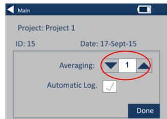
12 – To set the automatic logging, select the Automatic Log checkbox. This will save every measurement that is taken. Select Done when complete.
