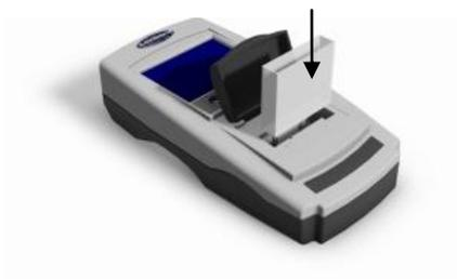
3 - Close the sample lid and press the test key on the keypad or the display.
