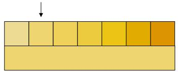
If the hue of the sample is dissimilar to the colour standards, making a match visually becomes far more subjective. In the diagram below, the nearest colour to the sample is shown by the arrow and it is this value that would be predicted by automatic instruments. Visually, because of the hue difference, the value selected might well be the next standard along to the right. The PFX*i* instrument would report this sample with an Off Hue factor of 5.
