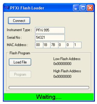
Click on the 'Load File' button and navigate to the new flash file ("PFXi\_100xx.flash"). The file will take a few seconds to load. When the file has loaded correctly, the 'Program' button will be enabled and the 'high' address of the firmware displayed (this is for information only):
