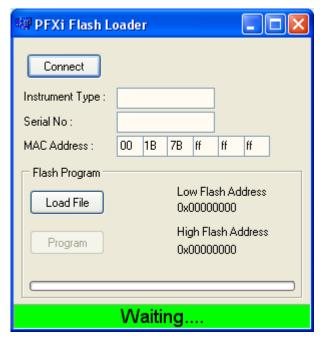
The green status bar indicates that the software is successfully communication with the instrument.
