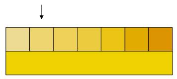
In the following example, the nearest colour is still the arrowed standard but Off Hue factor has been increased to 11. In this example one would expect a visual comparison to give the result as the 6<sup>th</sup> standard along.
