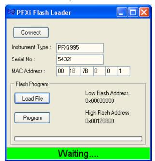
Click on the 'Program' button. The new firmware is then downloaded and programmed into the instrument.
