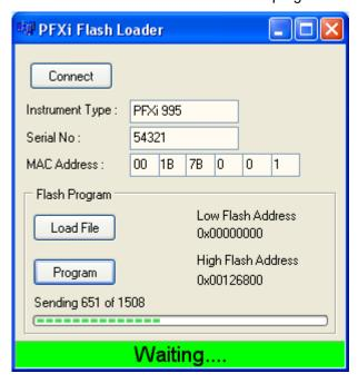
When programming is complete, the LCD screen will display 'Restart Instrument Update Successful' – Turn off the instrument power and restart. Confirm that the software version is correct on the instrument splash screen (it should match the version part of filename).
