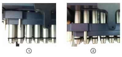
Figure 53 O-rings shown in a squeezed and relaxed state.
