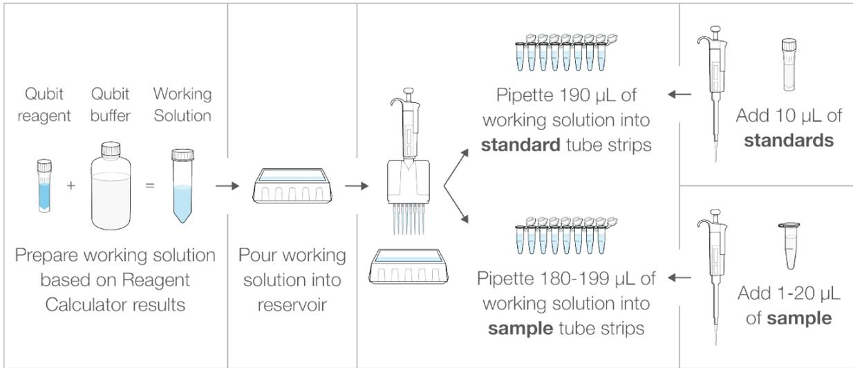
Figure 2 Overview of the Qubit™ RNA XR assay used with a Qubit™ Flex Fluorometer.
