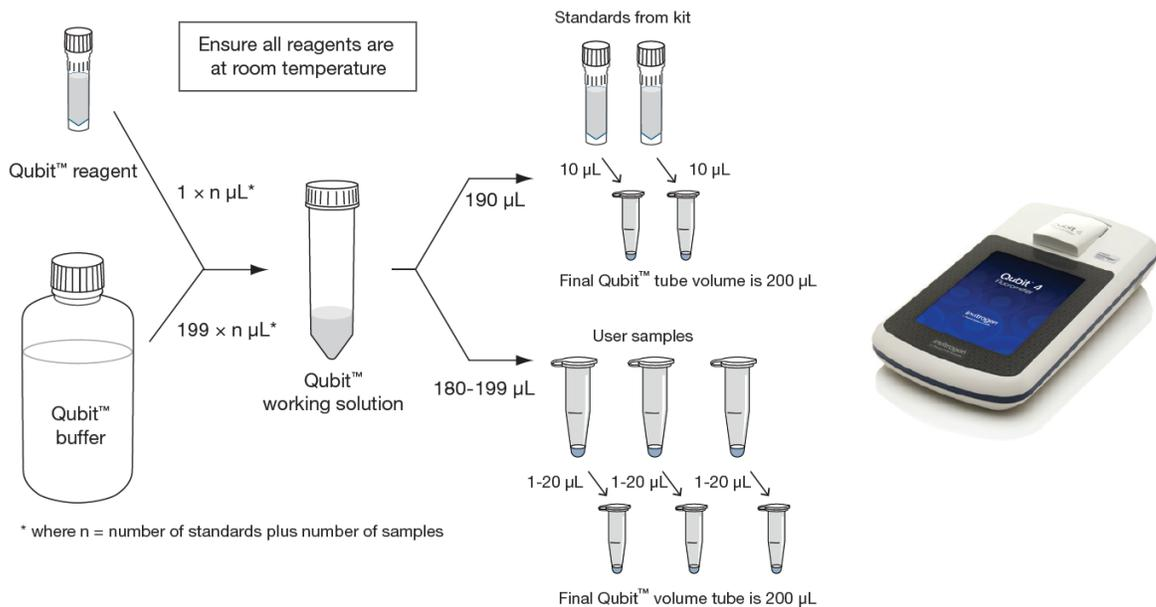
Figure 1 Overview of the Qubit™ RNA XR assay used with a Qubit™ 4 Fluorometer.
