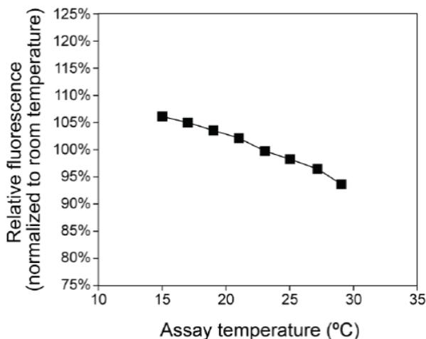
Figure 4 Plot of fluorescence vs. temperature for the Qubit™ RNA XR Assay.
