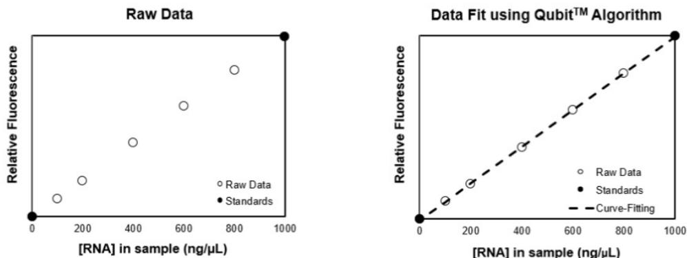
Figure 5 The curve-fitting algorithm used to determine concentration in the Qubit™ RNA XR Assay.
