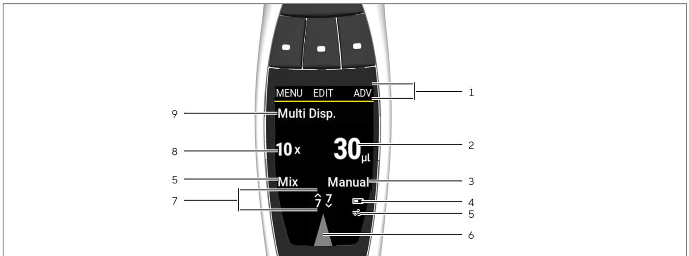
Fig. 5: Operating mode display (example)
