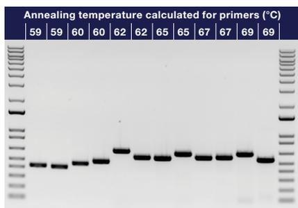
**Figure 2. PCR amplification with high specificity and yield following a universal annealing temperature at 60°C.** Primer sets with varying annealing temperatures were used to amplify 12 targets from human genomic DNA (gDNA) with a 60°C annealing temperature.
