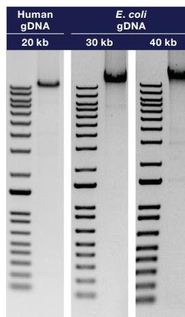
**Figure 5. Amplification of long fragments.** A 20 kb target from human gDNA and 30–40 kb targets from *E. coli* gDNA were successfully amplified by Platinum SuperFi II DNA Polymerase.
