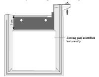
6. Hold the blot module together firmly and slide it into the guide rails on the lower buffer chamber. The blot module fits into the unit in only one way, such that the (+) sign is seen in the upper left hand corner of the blot module. The inverted gold post on the right hand side of the blot module fits into the hole next to the upright gold post on the right side of the lower buffer chamber.
