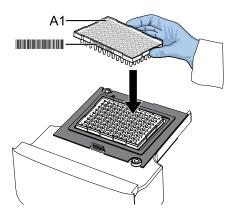
**Note:** Do not remove the black plate adapter before loading a plate or tube strips. If used, tube strips can fit loosely in the adapter, but the heated cover will apply the appropriate pressure to seat the tube strips securely in the adapter.
