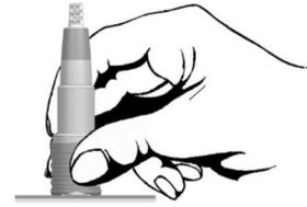
Now measurement and calculation of the coating thickness are carried out. This procedure takes approx. 1 second. Wait for the audible signal to confirm measurement has been completed. Then lift the sensor from the measuring object.
