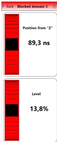
Blocking ranges are defined by the sliders for the position from the coupling echo Z and for echo amplitude in %.
