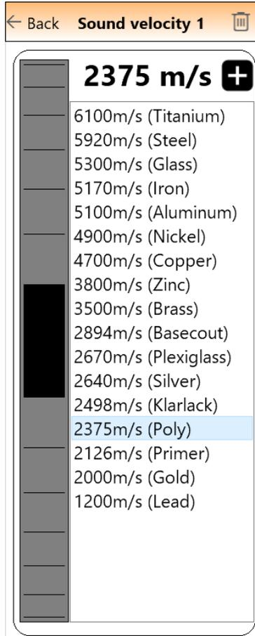
The corresponding configuration window, in this case Sound velocity 1.
