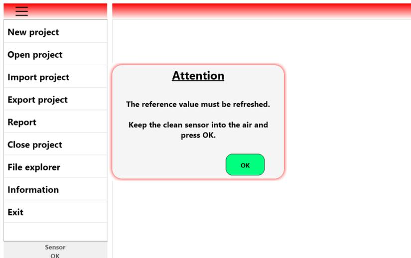
You will now be prompted to record a reference signal. Check the transparent measuring surface at the front of the sensor. There must be no impurities or residues of coupling agent on the measuring surface. If necessary, clean the measuring surface with water and a soft cloth.
