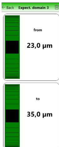
For each expected value, a tolerance band with a lower and an upper limit must be specified within which the respective layer thickness value should lie. When evaluating, these limits are always related to the position of the previous valid echo, meaning that only the current layer is considered, regardless of the thickness of previous layers and the position of the corresponding echoes.
