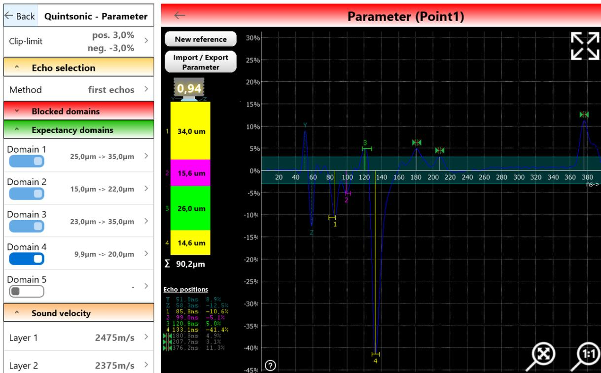
An expectancy domain is completely defined by its lower and upper limits (layer thickness values). In the A-scan, expectancy domains are indicated by horizontal lines in the width of the tolerance band. The assignment to the respective layer is determined by the position in Y-direction and corresponds to the layer thickness column on the left.
