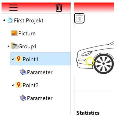
The designated measuring point can be marked on the photo or graphic inserted for a measuring point. A yellow circle is displayed.
