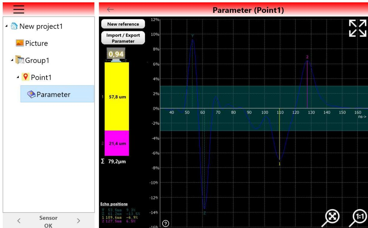
The signal contains a number of positive and negative impulses, including the coupling echo impulses and the echo impulses of the searched echoes at the layer boundaries.
