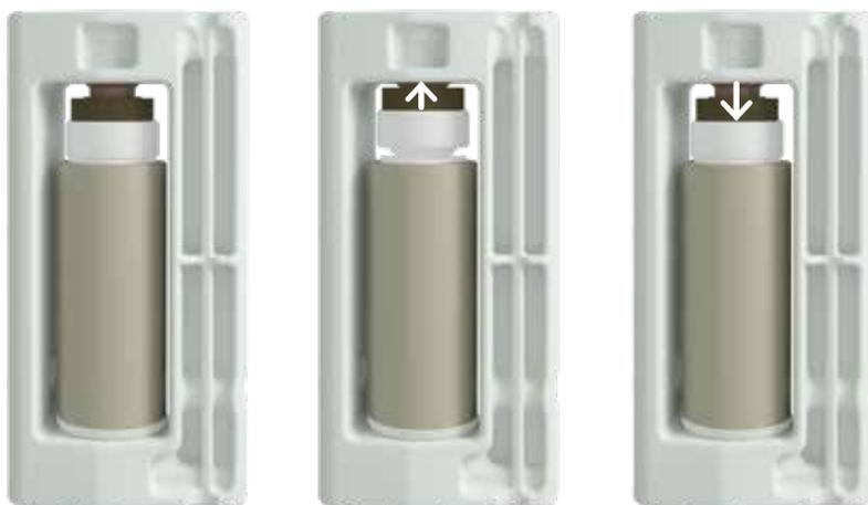
A safety spring built into the cover allows for precise venting of the vessel, if that should occur. Once the pressure has been reduced to a containable level, the cover closes again. Only the excess pressure, mainly generated by CO<sub>2</sub>, NO<sub>x</sub> fumes, is therefore released, allowing for a complete recovery of even volatile elements.
