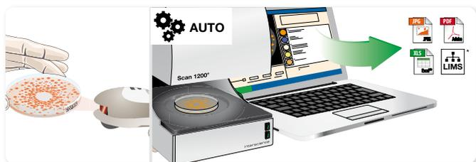
After incubation, scan the Datamatrix code. The **Scan**® colony counter is parametered automatically with the Datamatrix data. Click on "VALIDATE". Export the data.
