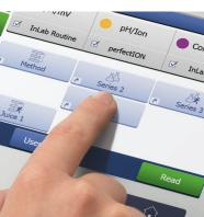
Start your own method, which is a sequence of analyses steps, with a single click. Using methods makes sure that your particular analysis is always performed with identical settings.
