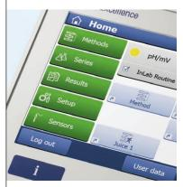
By a single click on a shortcut you can start a series or method. If started when running, the next analysis will be queued in the tasklist and starts automatically upon completion of the previous task.
