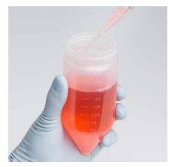
Nunc 200 mL and 250 mL Conical Centrifuge Tubes offer added capacity for your larger samples. The 250 mL (shown) has a unique, wide-mouth design that provides easy access for pipetting, decanting, and removal of pellets following centrifugation.
