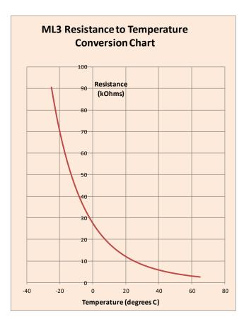
Note: This table has been optimised for use as a look-up table. To minimise linear interpolation errors the data points fall either side of the manufacturers' specified sensor response curve. This helps optimise the overall accuracy of readings.
