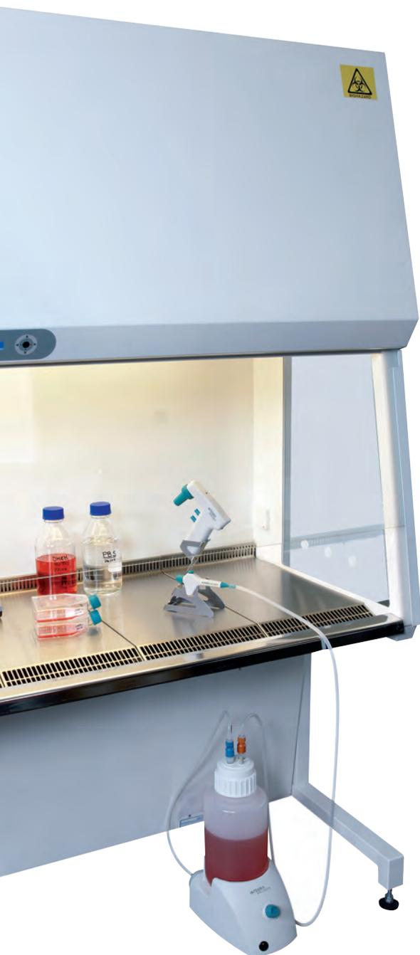
Vacuum systems are widely used for aspiration of liquids and their subsequent disposal. Common applications include the removal of media from cell cultures, of supernatants after centrifugation and of wash solutions from immuno-assay well-plates.
