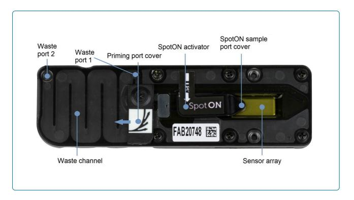
**Slide open the priming port cover and gently lift open the SpotON sample port cover.**
