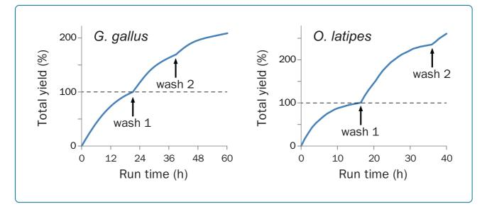
**Figure 3.** Throughput observed from *Gallus gallus* and *Oryzias latipes* libraries run on a PromethION Flow Cell and a MinION Flow Cell, respectively. The arrows indicate the timing of each wash step: wash steps were performed at the point where the rate of data acquisition started to slow due to the accumulation of "recovering" pores. In each case, output is more than doubled from the point of the first wash.
