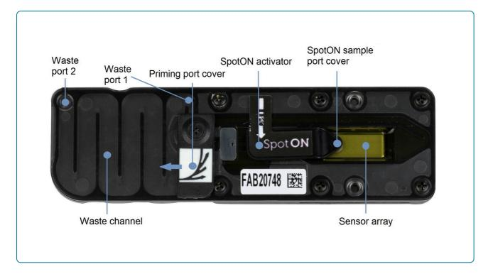
**10** Slide the flow cell priming port cover clockwise to open.
